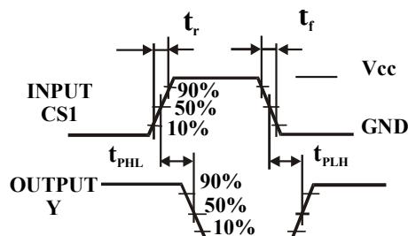
Figure 1. Switching Waveforms
