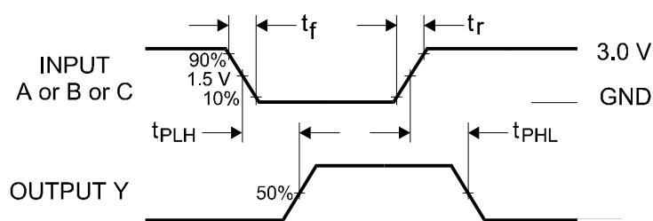
**Figure 1. Switching Waveforms**
